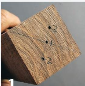
Mark the true center and label it 1. Then add two other axis points  $\frac{1}{2}$ " away, labeled 2 and 3. Do this on both ends of the blank.
