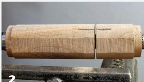
Rough-turn the blank and turn tenons on both ends. Make a partial parting cut where the lid and bottom will be separated and finish the cut off the lathe. Make a reference mark for future alignment.
