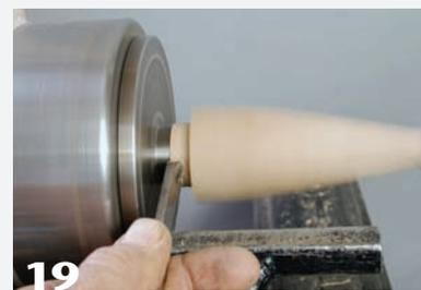
The box is mounted on expanding pin jaws to refine the tight fit of the lid. Use a sharp parting tool to lightly trim the tenon until you reach your desired fit.
