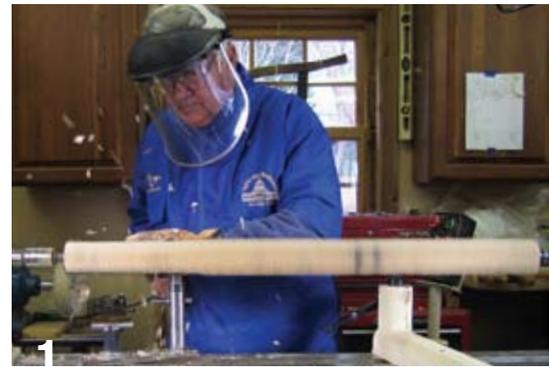
Mount a kiln-dried 2x2x37" blank between centers. (Hardwoods such as maple, walnut, oak, and ash work best.) Using a spindle roughing gouge, C. A. Savoy brings the bottom half of the cane into round by working from the tailstock toward the headstock.
