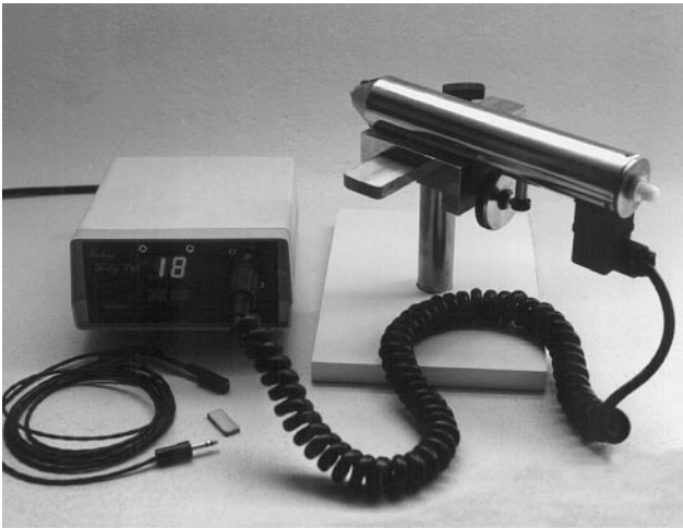
The RS3000 consists of a microprocessor/sensor and magnet system. Together, they monitor lathe speed and control a solenoid-driven cutter mounted in a conventional tool-rest base. At right is a small sampling of the range of decoration the system is capable of.
